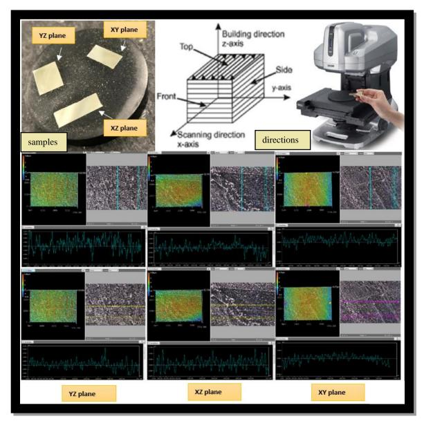
Figure 3: 3D surface finish and deviations in micrometers
