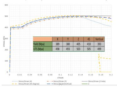
STRESS/STRAIN (DEPOSITION ALONG DIFFERENT AXIS)
