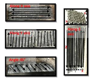
**Figure 12:** Hybrid 3D printing layers' directions: along X axis, across Y axis, at angle 45°, and vertical Z axis.
