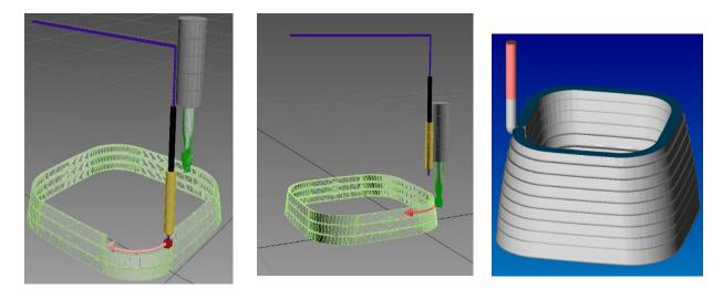
Figure 1: 3D metal printing (left) and machining processes
